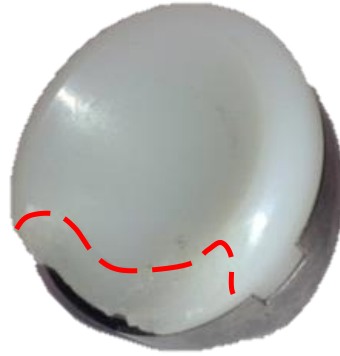
Figure 2-1: Retrieved humeral cup with advanced defect from scapular notching highlighted (red outline)
